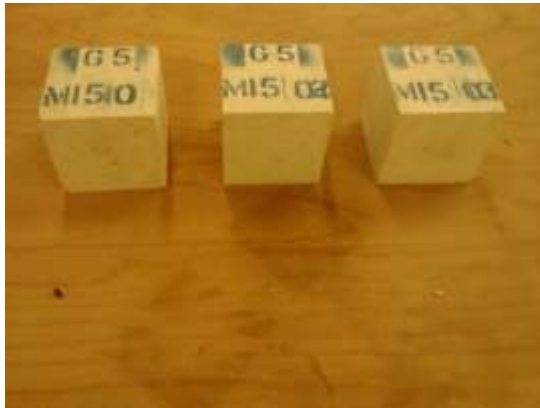
Figure 6: Labelling of concrete cubes for quality control
