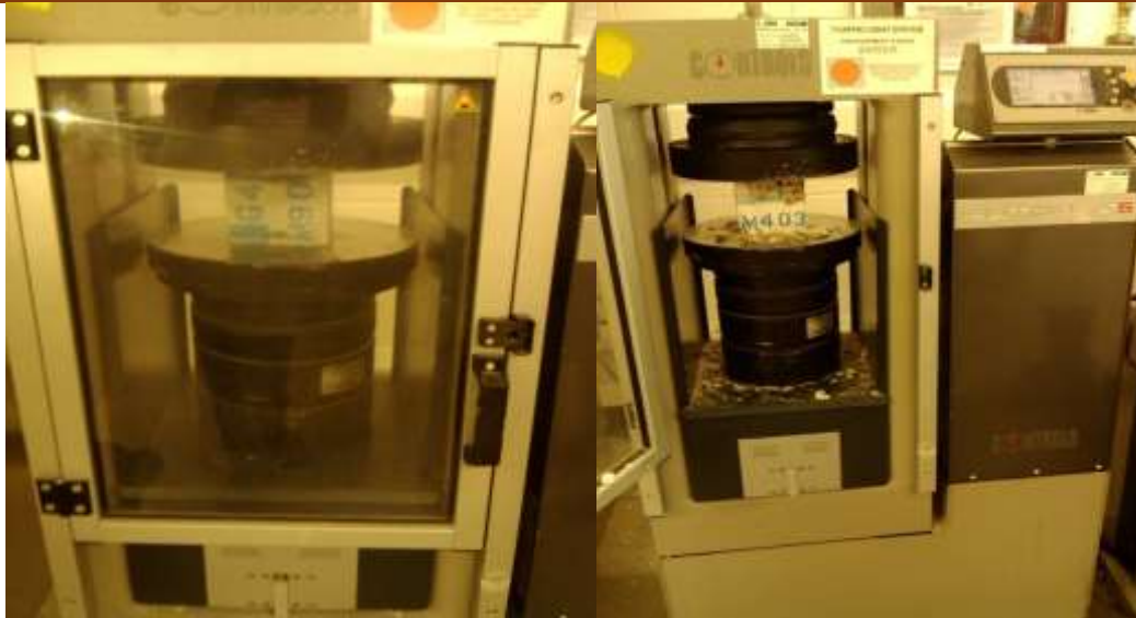
Figure 5a: Concrete cube during testing
