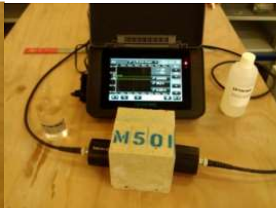
Figure 7: Proceq pulse velocity machine test in use
